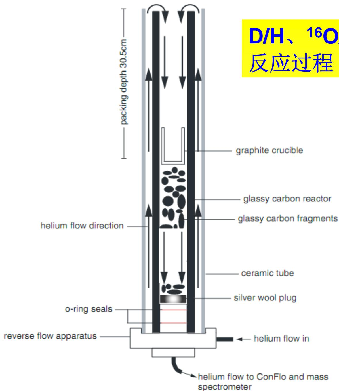
to scale) of the 'reverse-plumbed' TC/EA reactor showing the flow of He carrier gas. The purpose of the
